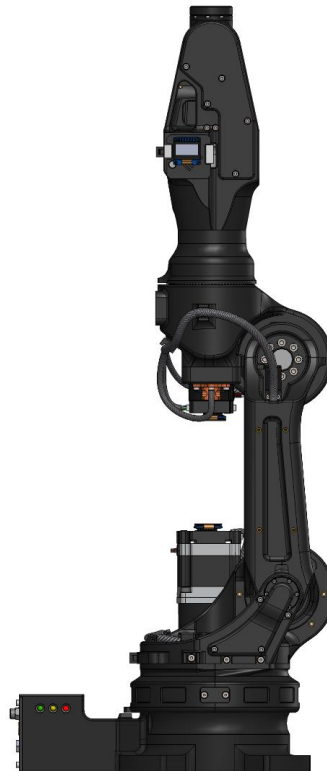
Zero position of the Astorino robot arm.
